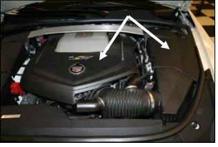
1. **Disconnect the negative battery cable.** Remove the engine and shock tower covers by simply pulling up on them and sliding out from the vehicle. These will be reused later in step 14.
