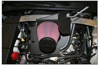
**10.** Install the Bracket (#27) on to the Rear Panel (#4) as shown using one 1/4-20 Button Head Screw (#19), 1/4" Flat Washer (#18), and 1/4" Serrated Nut(#20). Complete the assembly by attaching the Airaid Premium Filter (#1) to the Filter adapter (#8).
