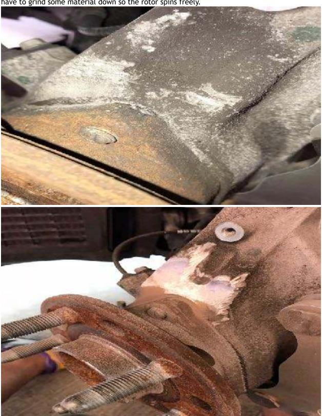
Finished product. Make sure to use Red or Blue Loctite on all fasteners. Make certain to check for leaks once brake lines are attached.
