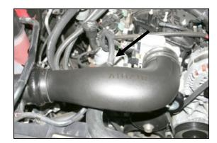
12. Install the Airaid Intake Tube into the hump hose first, and then onto the throttle body. Adjust it for fit, and tighten the hose clamps. Next install the 3/8" x 14" breather hose (#8) between the 1/4" NPT x 3/8" barbed fitting in the tube, and the factory port on the valve cover.
