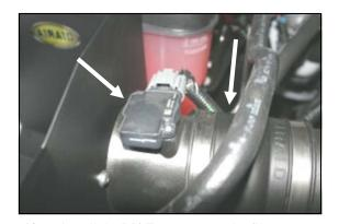
10. Reinstall the MAF sensor onto the filter adapter using two 8-32 x 5/8" Allen Bolts (#13). Do Not Use The Factory Screws! Next install the urethane hump hose (#6) onto the **MAF** with the two #64 hose clamps (#17).
