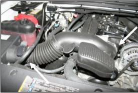
**4.** Loosen two hose clamps on the factory intake tube. One at the throttlebody, and one where it clamps to the factory airbox. Remove the factory
