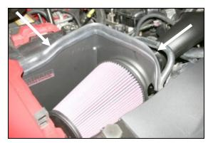
13. Install the Airaid Premium Filter (#1) onto the air filter adapter, and tighten the hose clamp. Next install the provided weather strip (#9) onto the top of the CAD. For ease of install, start at the inner fender, and work your way towards the radiator. Reinstall the beauty cover.
