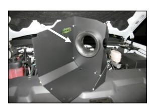
**8.** Assemble the Cool Air **D**am panels (**CAD**) (#2 & #3) using five 6-32 x 5/16" screws (#10), #6 flat washers (#11), and 6-32 keps nuts (#12). Next install the air filter adapter (#5) into the panels as shown with the hole for the **M**ass **Air Fl**ow sensor facing up, using three 1/4 - 20 x 1/2" button head bolts (#14), and 1/4" flat washers (#15). Apply the Airaid Foil Decal onto the Panel as shown.
