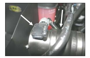
**10.** Reinstall the **MAF** sensor onto the filter adapter using two 8-32 x 5/8" Allen Bolts (#13). **Do Not Use The Factory Screws!** Next install the urethane hump hose (#6) onto the **MAF** with the two #64 hose clamps (#17).
