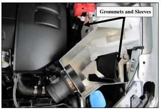
11. Install the Air Dam assembly into the inner fender area of the vehicle in the same manner as the OEM airbox. The grommets and sleeves are to be secured to the inner fender by re using the 6mm nuts that were removed in step Three.
