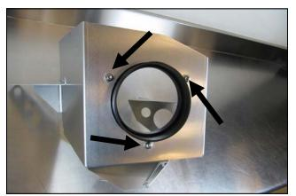
**6.** Carefully remove the protective film from both sides of the Air Dam. Install the Filter Adapter onto the Air Dam as shown using the three Button Head Screws and Flat washers.
