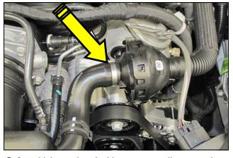
**5.** On vehicles equipped with a resonator, disconnect the tube at the diaphragm and block off the inlet using the supplied Cap.
