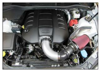
Double check your work! Make sure there is no foreign material in the intake path. Make sure all clamps, hoses, bolts, and screws are tight. Double check the hood clearance. Reconnect the negative battery cable.
