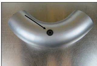
14. Insert the Grommet into the Airaid Intake Tube a shown.
