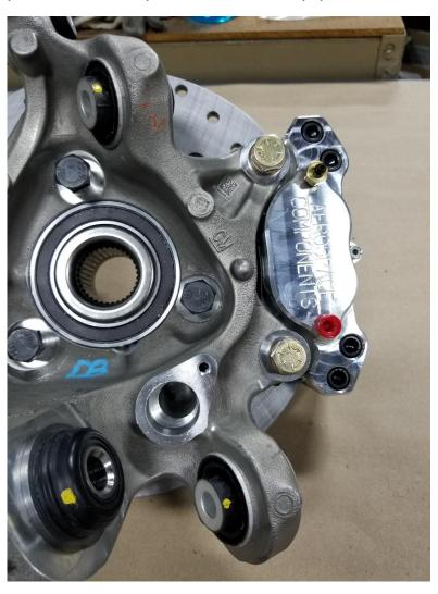
\*Drop the pads into the calipers with the friction side facing the rotor and secure them with the pad retaining bolt and ny-lock nut. Be sure the bolt extends through the locking feature of the nut and tighten until you can barely spin the pad bolt with your fingers. Make sure the brake pads are the only thing touching the rotor! The rotor should be centered in the caliper.
