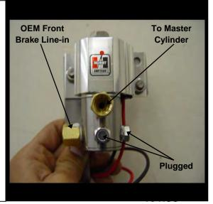
4. Ensure that the new brake line routing is understood prior to installation. However, DO NOT attach lines to solenoid at this time.
