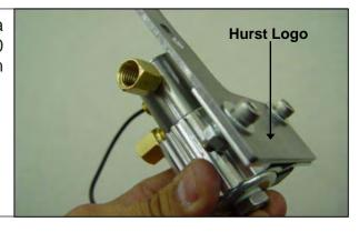
3. Tighten the provided adapters and plugs to solenoid as shown.
