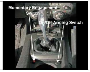
12. Reconnect battery and turn ignition switch to the "ON" position. While still in park and NOT depressing your brake pedal, activate and engage your Hurst Roll/Control system (make sure you can hear the clicking of the solenoid) several times and check fuse. If fuse is burned, check all electrical connections for a short and correct any problems immediately.
