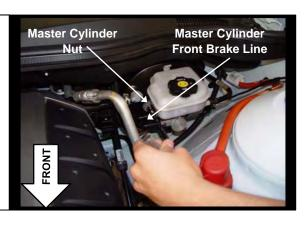
6. Install the Hurst Roll Control brake line to solenoid, however, do not completely tighten fittings at this time to allow for minor adjustments.
